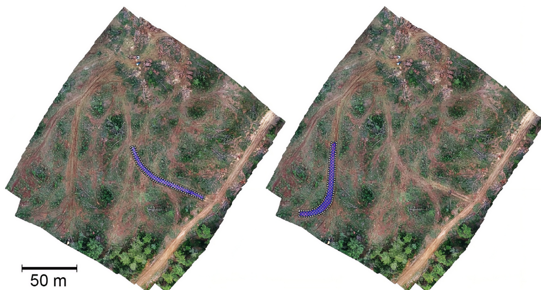
Figure 3: Skidding roads for 0-20% (left) and 20-50% (right) slope groups.
