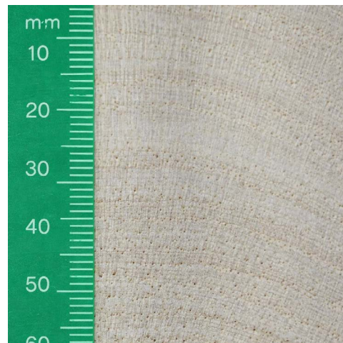
Figure 3: Sanded surface of Erythrina poeppigiana wood. Scale in mm.
