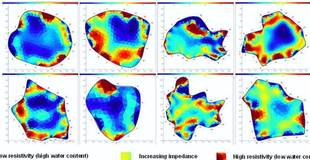
**Figure 4:** Individuals of *Spathodea campanulata* exhibiting internal deterioration in the central trunk section, as observed through Electrical Resistance Tomography (ERT).
