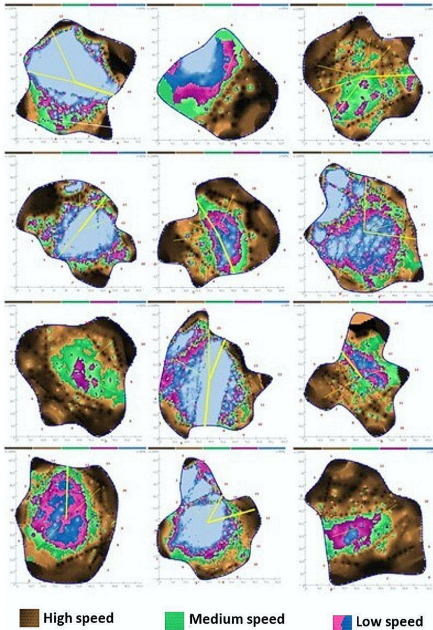
**Figure 2:** Measurements of the trunk sections of *Spathodea campanulata* individuals exhibiting prominent internal condition defects using sonic tomography (SoT).
