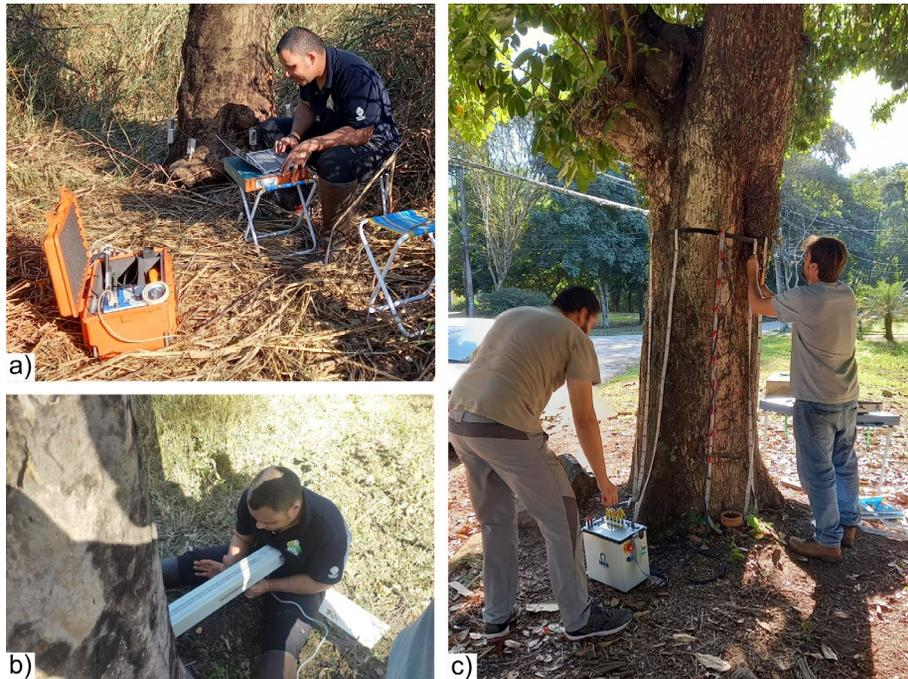
**Figure 2:** Data acquisition with proposed methodologies. a) Mechanical impulse tomograph. b) Resistograph. c) Electrical resistivity.
