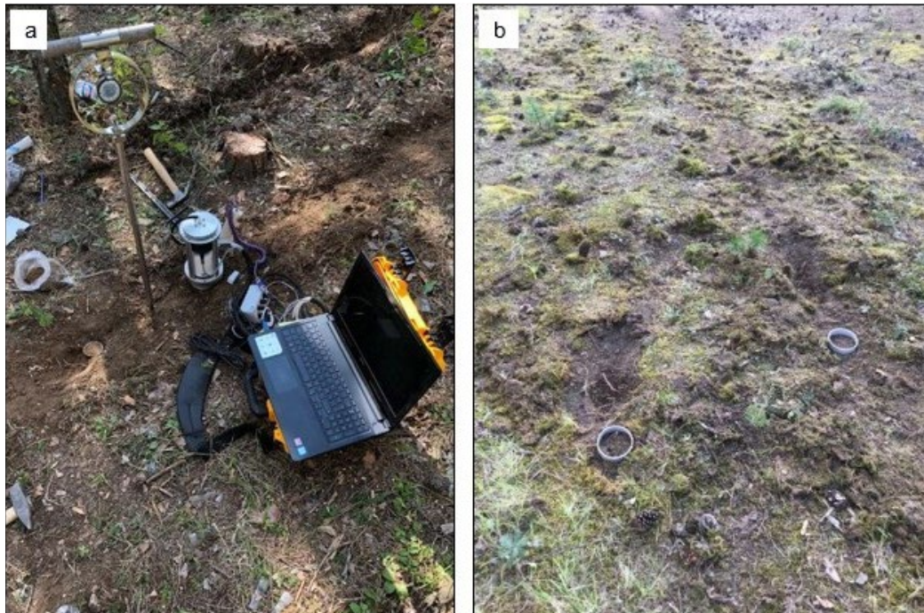
Figure 2: Shows soil respiration measurement studies after harvesting operations. (a) Soil respiration measurement method; (b) soil respiration measurement points.
