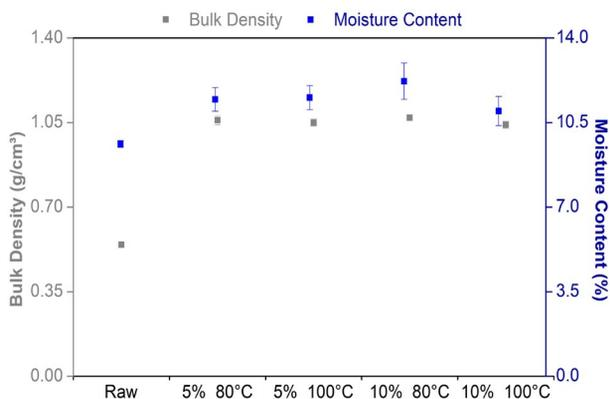
**Figure 5:** Bulk density and moisture content of the patauá fibers: raw, treated with NaOH at 5% at 80°C, treated with NaOH at 10% at 80°C, treated with NaOH at 5% at 100°C, and treated with NaOH at 10% at 100°C.
