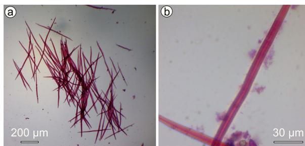
**Figure 2:** Optical micrographs of macerated patauá fibers: (a) general view, and (b) lumen and cell wall.
