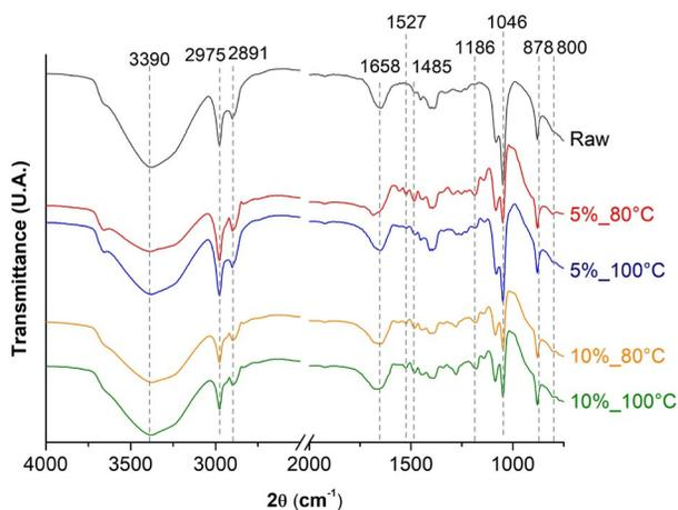
**Figure 4:** FTIR spectra of the patauá fibers: raw, treated with NaOH at 5% at 80°C treated with NaOH at 10% at 80°C, treated with NaOH at 5% at 100°C, and treated with NaOH at 10% at 100°C.
