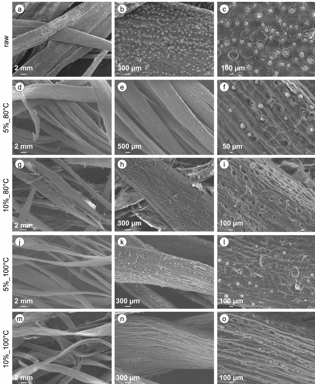
**Figure 3:** SEM micrographs of the patauá fibers: (a-c) raw, (d-f) treated with NaOH at 5% at 80°C, (g-i) treated with NaOH at 10% at 80°C, (j-l) treated with NaOH at 5% at 100°C, and (m-o) treated with NaOH at 10% at 100°C.
