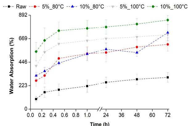
**Figure 6:** Water absorption of the patauá fibers over time: raw, treated with NaOH at 5% at 80°C, treated with NaOH at 10% at 80°C, treated with NaOH at 5% at 100°C, and treated with NaOH at 10% at 100°C.
