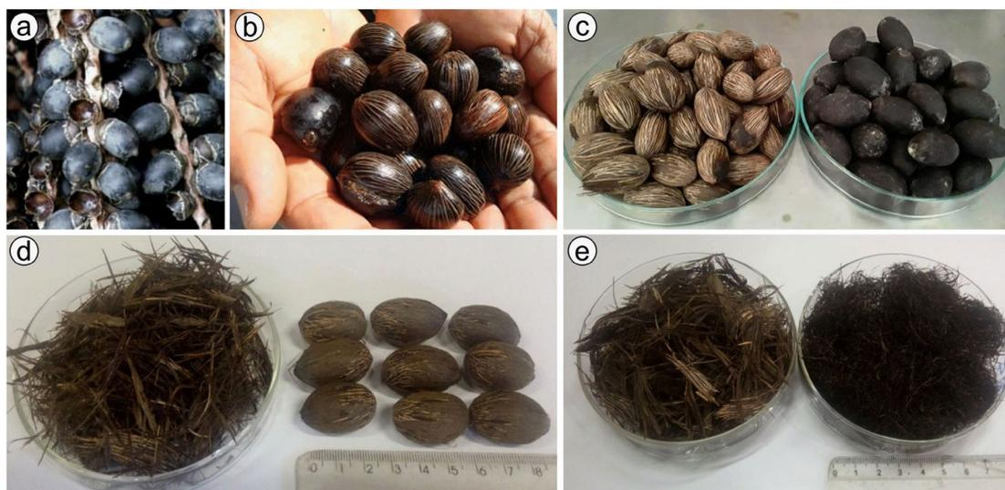
**Figure 1:** From the fruit to the thermochemically treated patauá fibers: (a) fruit brunch; (b) harvested fruits; (c) depulped seed waste (left) and fruit (right); (d) raw fibers (left) removed from the surface of the seeds (right); (e) raw fibers (left) and fibers treated with 10% of NaOH at 100°C.
