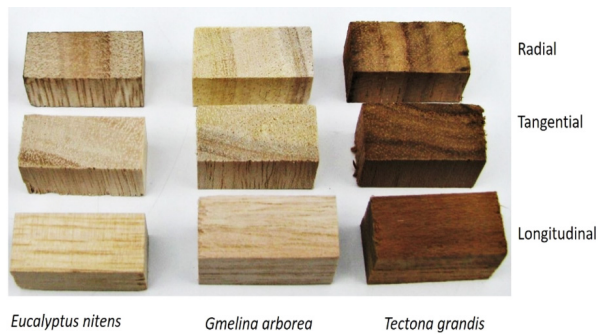
FIGURE 2 Samples of the three different woods in the longitudinal, tangential and radial directions.
