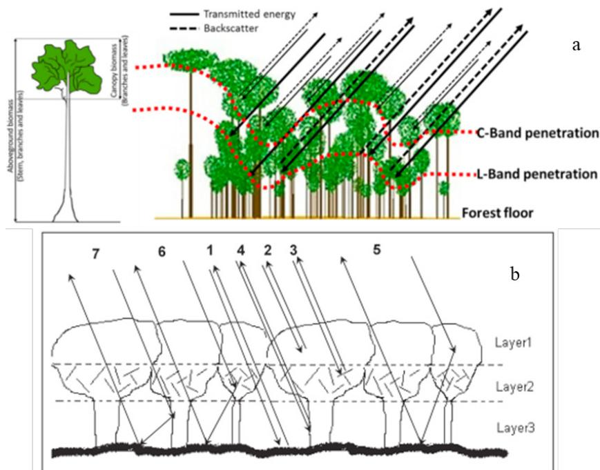
**FIGURE 1** (a) Penetration of the C and L bands wavelength in the forest canopy. Source: (OMAR et al., 2017). (b) Geometry of a forest canopy and scattering components: 1, soil surface scattering; 2, leaf volume scattering; 3, branch volume scattering; 4, trunk volume scattering; 5, leaf-soil interaction; 6, branch-soil interaction; 7, trunk-soil interaction. Source: (WANG and QI, 2008).
