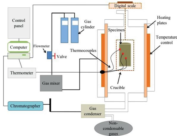
**FIGURE 1** Design of Macro ATG oven plant.
