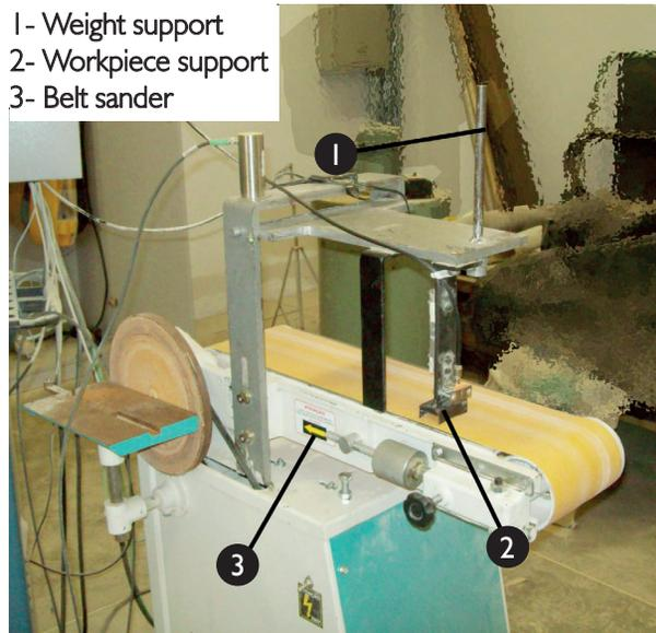
FIGURE 1 Belt sander used in the experiment.
