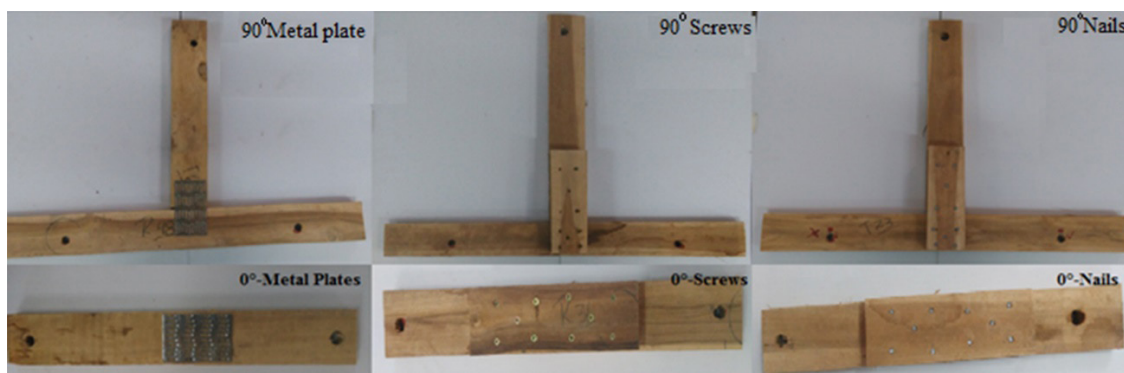
FIGURE 1 Orientation of truss connections and distribution of metal plates, nails and screws.
