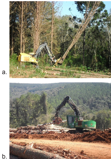
FIGURE 1 Feller buncher (a) and harvester (b) evaluated in a clearcutting operation of pine stand.
