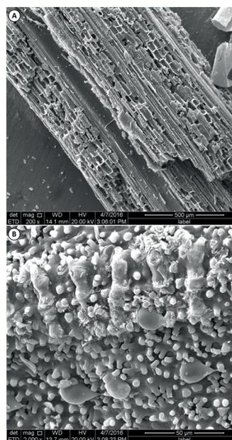
**FIGURE 4** Surface morphology of  $H_3PO_4/H_2OAC$  obtained by scanning electronic microscopy for a 20 kv tension. Presence of an organized pore network (A) and regions with protuberances in the wall of the fibrovascular bundle of  $H_3PO_4/H_2OAC$  (B).
