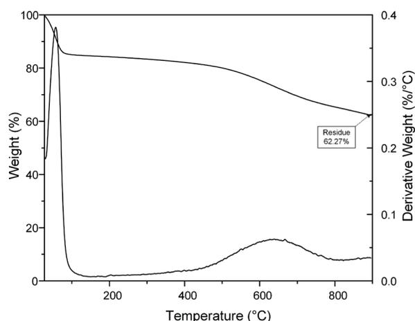
FIGURE 2 Thermogravimetric analysis for the produced H<sub>3</sub>PO<sub>4</sub>/H<sub>2</sub>OAC.
