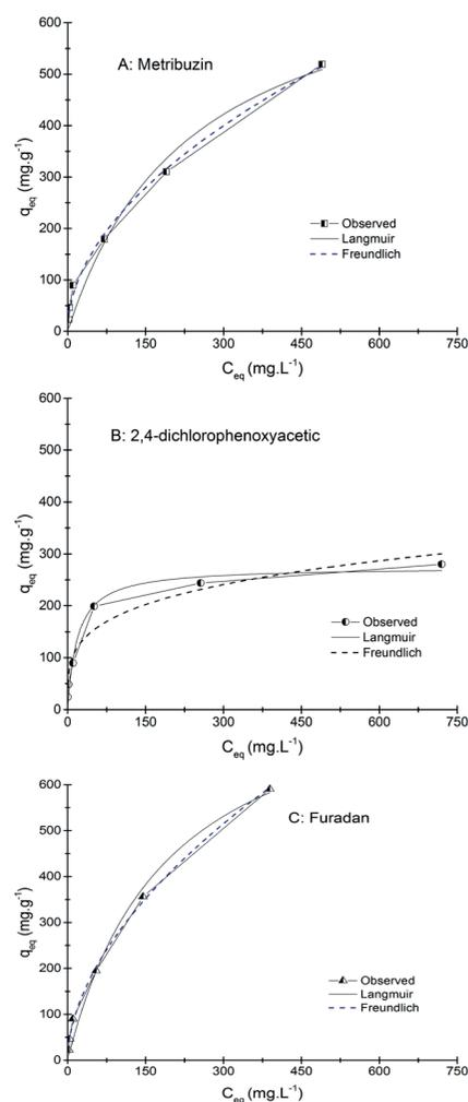
**FIGURE 5** Adsorption isotherms for the pesticides (A) metribuzin, (B) 2,4-dichlorophenoxyacetic and (C) furadan for the produced AC (10 mg of AC; 10 mL of different solution concentrations; 25 °C; q<sub>eq</sub> = adsorbed contaminant quantity; C<sub>eq</sub> = balance concentration).
